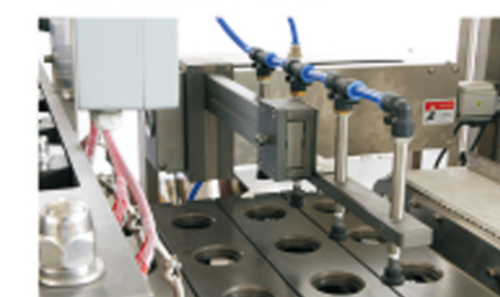
9. Finished capsule sucking to conveyor
